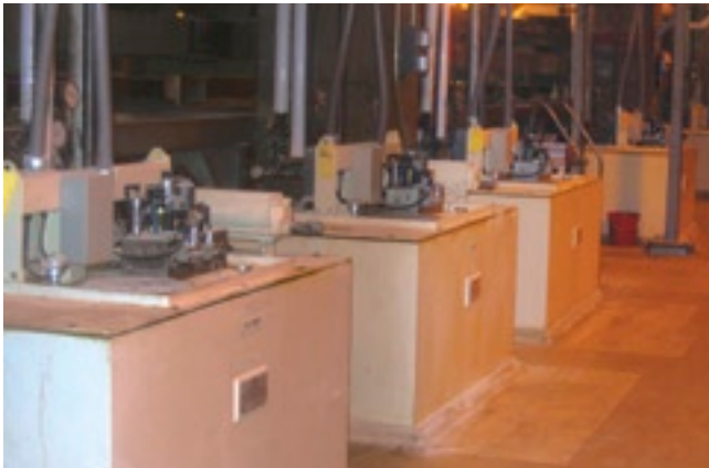
Hershey Chocolate of Virginia, Inc. called upon Petro-Canada to perform a plant lubrication analysis and assist in the complete conversion and consolidation to PURITY FG lubricants. Shown here are Duyvis peanut press hydraulic systems – lubricant in use is PURITY FG AW Hydraulic Fluid 68.
